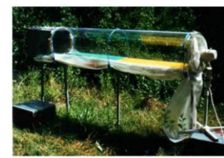
Figure 4. Wind tunnel study of neonicotinoid toxicity. 20 bees were tested in the wind tunnel with a flow of 1 m/s.
