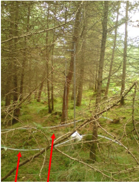
Network of gas release lines laid across woodland floor
