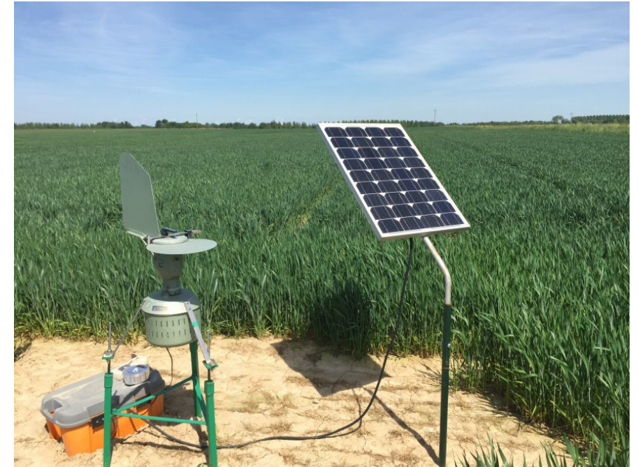
Burkard 7-day volumetric spore sampler
