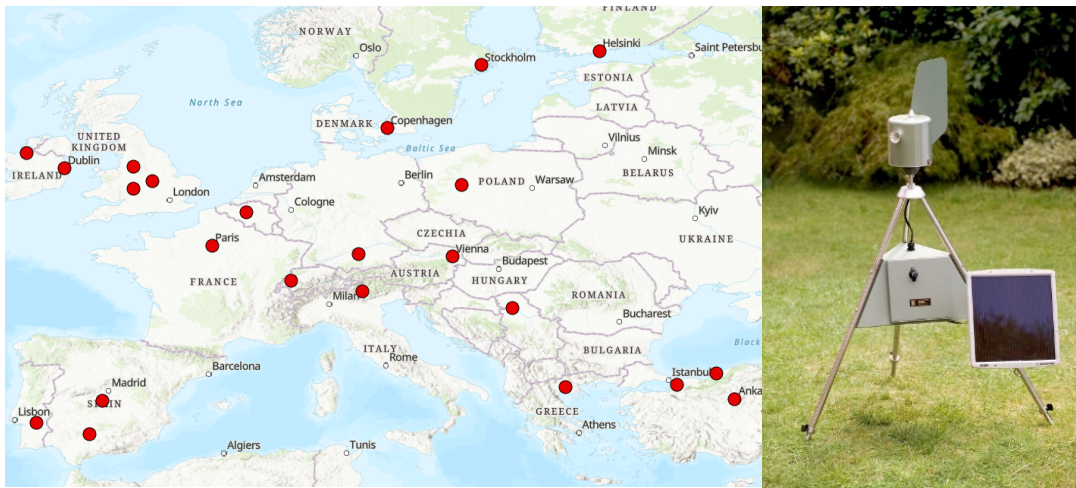
Figure 1. COST ADOPT campaign as executed in 2024. Left: Location of sites. Right. Multi-vial dry cyclone used for collecting material.
